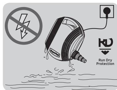
The pump has a thermal overload safety device. In the event of any overheating of the motor, this device automatically switches off the pump. The cooling time is roughly 15 to 20 minutes, then the pump automatically comes on again. If the overload cutout is tripped, it is essential to identify and deal with the cause of the overheating.
