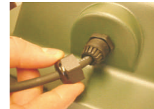
2). Loosen cable gland and push some excess cable through.
