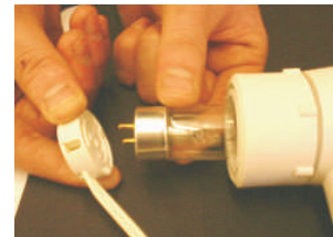
5). Disconnect lamp holders and remove lamp
