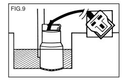
When submersing or lifting the pump it will be necessary to use a rope or chain, this must be attached to the transport handle.
