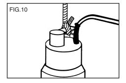
If pumping water from a sandy or muddy floor bed, the pump can be suspended using a rope or chain (not supplied) fixed to the handle. DO NOT use any of the electrical cables for this purpose.
