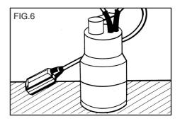
When the float switch reaches the minimum level it will automatically switch the pump off.
